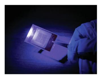
To enable the development of wearable devices that possess advanced ultraviolet (UV) detection functions, scientists from Nanyang Technological University, Singapore (NTU Singapore) have created a new type of light sensor that is both flexible and highly sensitive.
